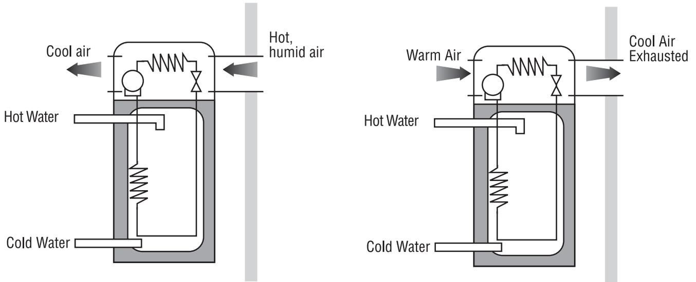
**Summer:** Hot and humid outside air is drawn in past the unit and cool, dry air is fed into the house ventilation system.
